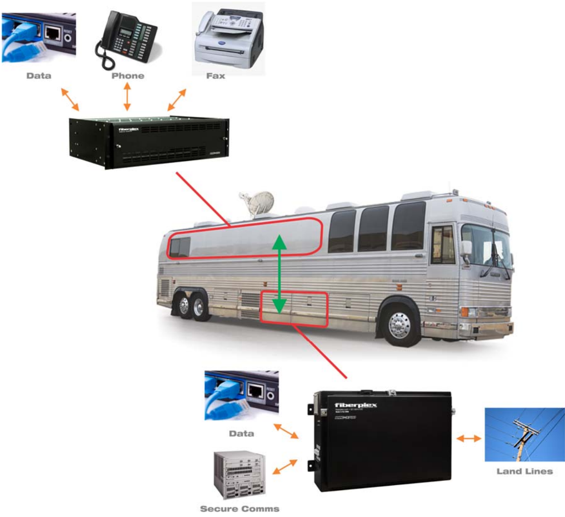
Figure 1 Block diagram of FiberPlex comms in Mobile Command Center
